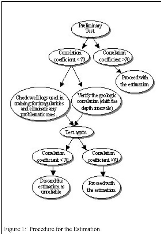
Figure 1 shows the procedure to be followed for the estimation. Once the data gathering is carried out, it is convenient to execute some preliminary tests to verify the quality of the estimation.
