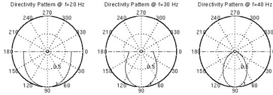
Figure 1: A Six Geophone Array Directivity Pattern.
