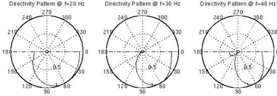
Figure 3: Six Geophone Array Directivity Pattern with Shifting.
