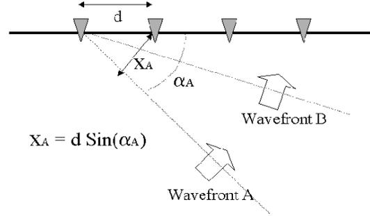
Figure 4: Directional Array Filter Design.
