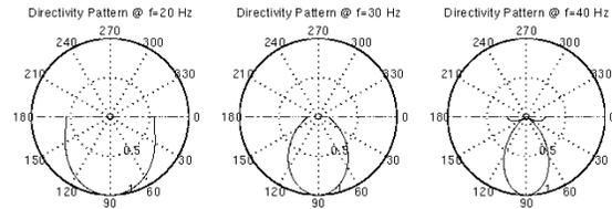
Figure 2: Six Geophone Array Directivity Pattern with Weighting.
