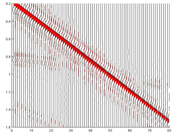
Figure 10: Processed Seismic Section with the Horizontal Reflection Cancelled.
